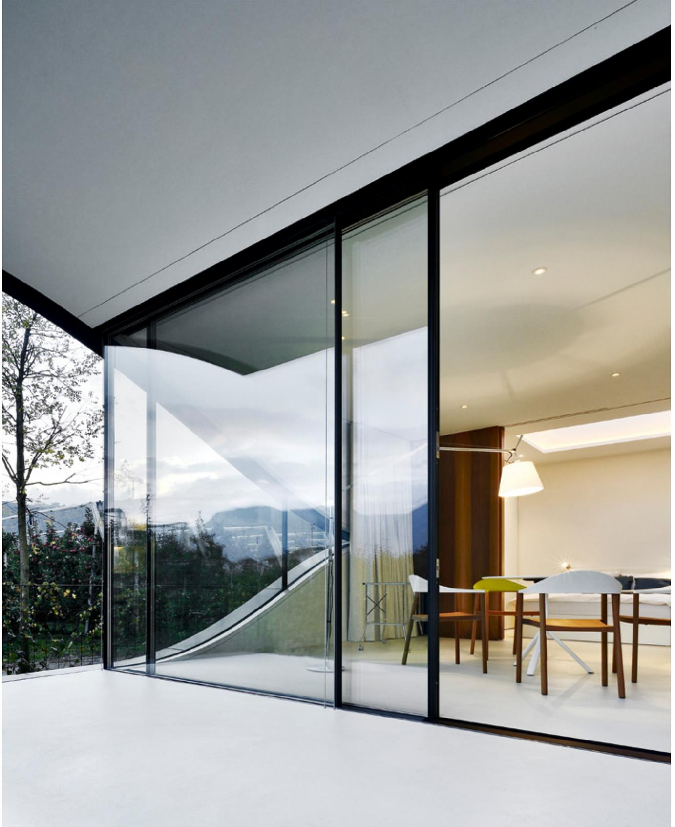
Sky-Frame Drive's electric drive facilitates simple and virtually noiseless operation of up to 6 (3+3) sliding panels at the press of a button. The drive is concealed in the ceiling section and allows the window panels to move automatically.
